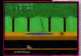
[Atari 2600] Early consoles only output RF video – tremendously noisy and fuzzy, but details weren't fine enough to be lost.
